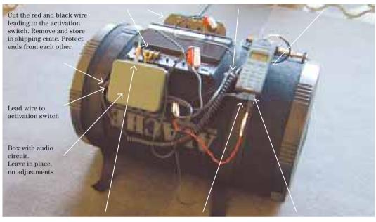
9-12 v dc Tip is positive (+) Can use standard wall adaptor
